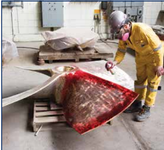
Dye Penetrant Testing for Propeller
